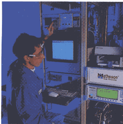
APIMS used for valve experiments.
