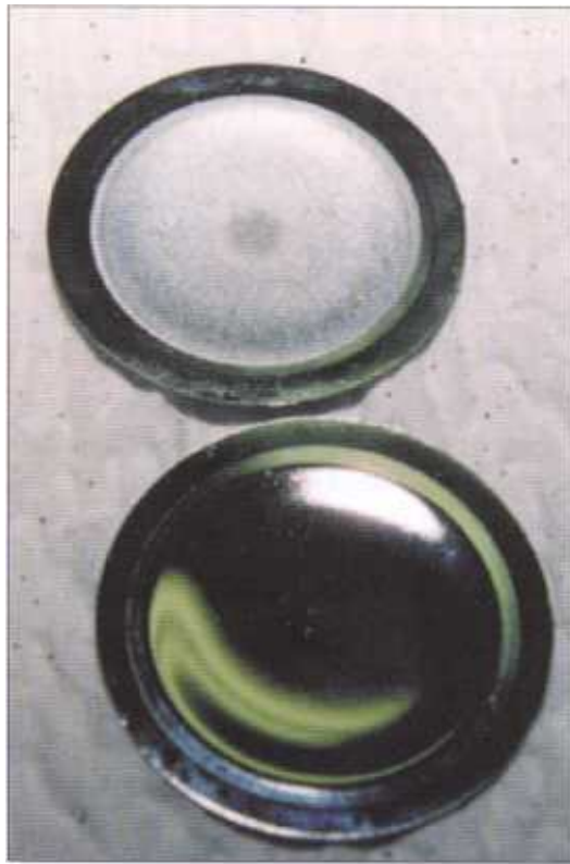
Figure 10 Wetted surfaces of upstream (top) and downstream (bottom) valve diaphragms from a purifier that was in HBr service for three years
