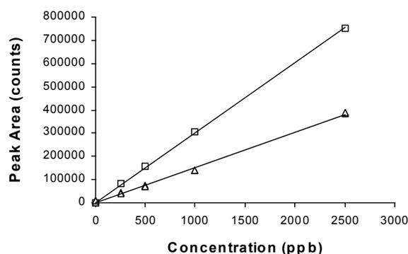
Figure 5. Calibration curves for CO<sub>2</sub> in He (□) and NH<sub>3</sub> (Δ) matrices.
