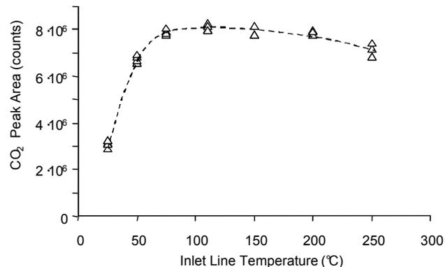
Figure 4. Effect of manifold temperature on free CO<sub>2</sub> response in ammonia
