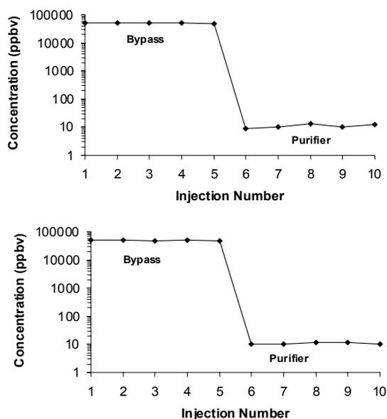
Figure 6. Efficiency experiment showing removal of 50 ppmv CO<sub>2</sub> in ammonia by NHX-Plus, Upper graph: removal of free CO<sub>2</sub> (zones 1 and 2 heated to 110°C). Lower graph: removal of complexed CO<sub>2</sub> (zone 1 unheated and zone 2 heated to 110°C).
