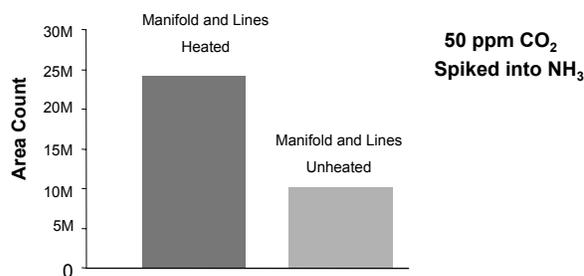
Figure 3: Free CO<sub>2</sub> in NH<sub>3</sub> measured with heated (145°C) and unheated manifold and lines.
