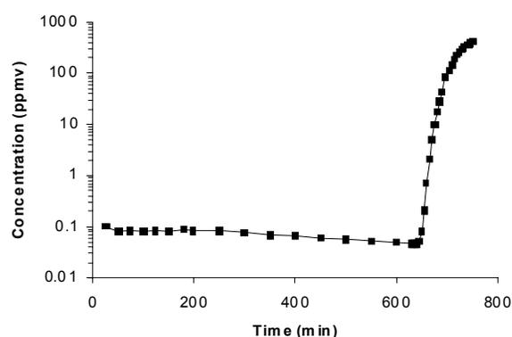
Figure 7. NHX-Plus purifier capacity experiment showing CO<sub>2</sub> removal to <50 ppb and breakthrough at 660-665 minutes. Challenge: 500 ppmv CO<sub>2</sub> in helium at 1 slpm.
