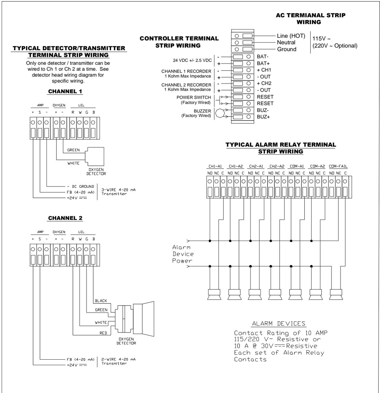
**Figure 5: Terminal Strip Wiring Connections**
