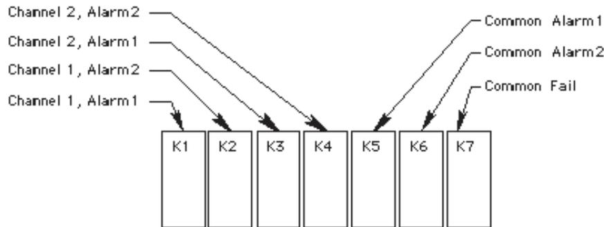
Figure 3. Beacon 200 Channel Relay Allocation
