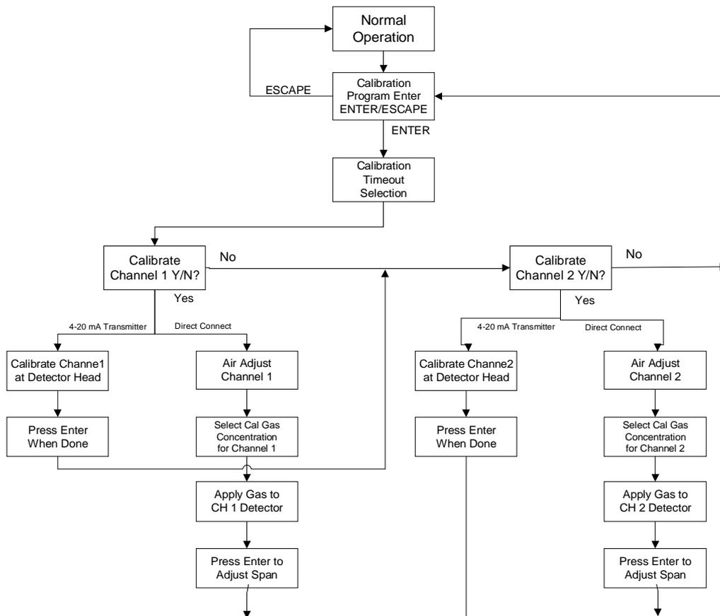
Figure 13: 4-20 mA & Direct Connect Detector Head(s)
