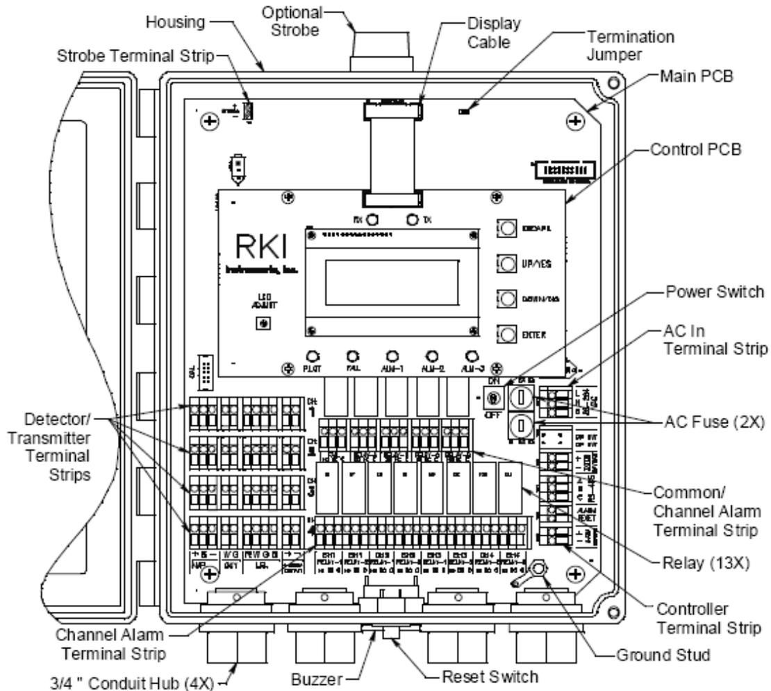
Figure 1: Beacon 410 Gas Monitor Component Location
