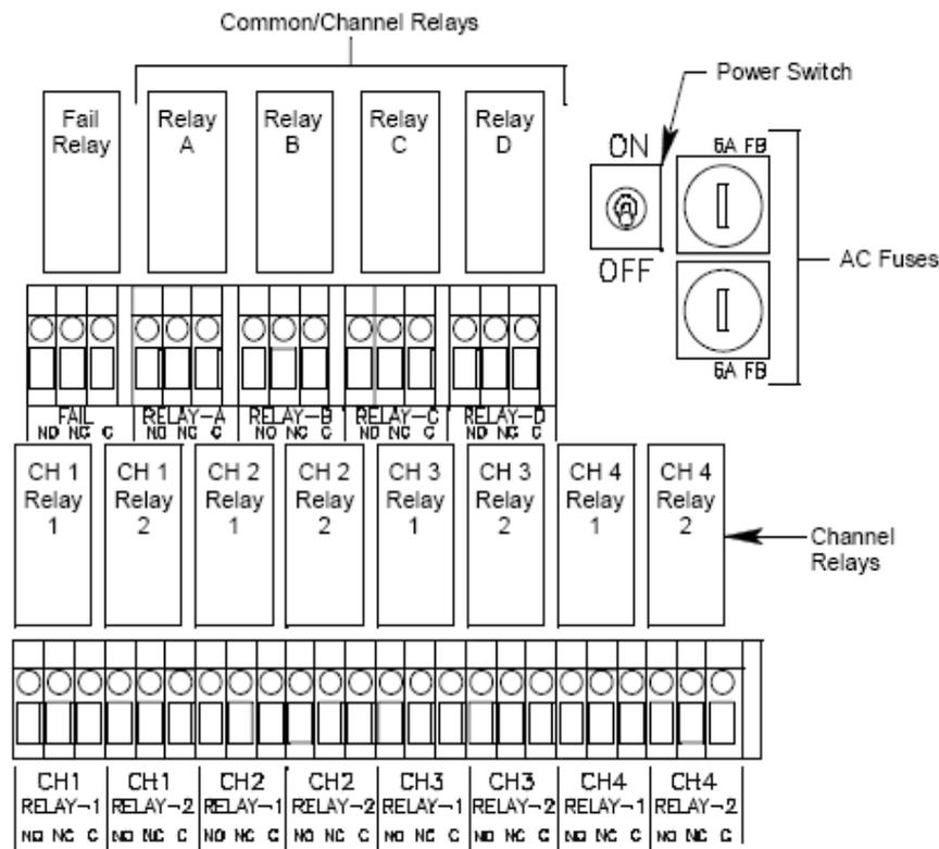
Figure 3: GasScanner 4C Relay Allocation
