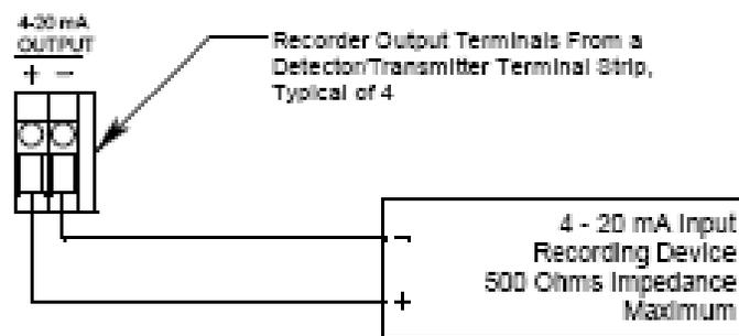
Figure 9: Recorder Output Wiring
