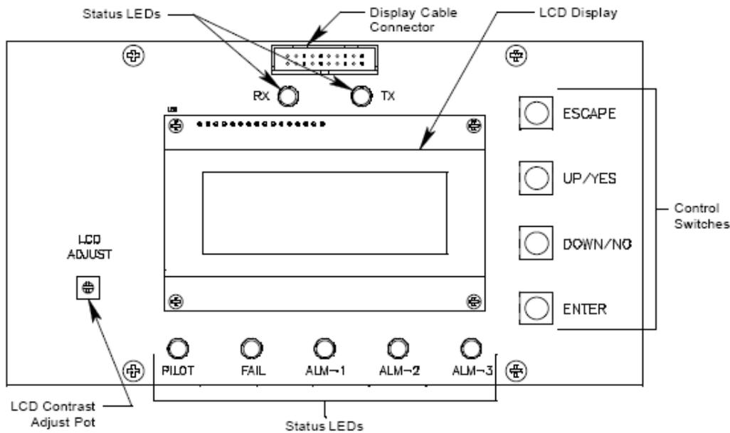
Figure 2: Control PCB Component Location
