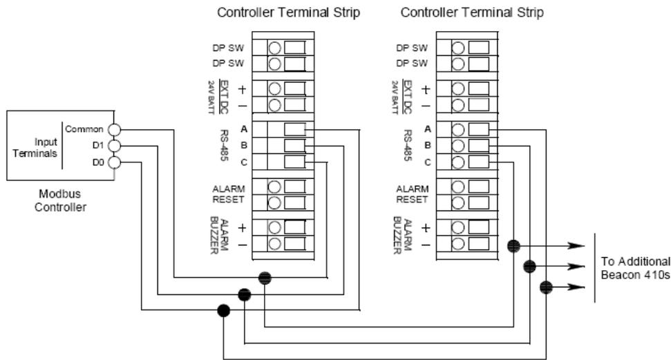
Figure 11: Recommended Modbus Wiring
