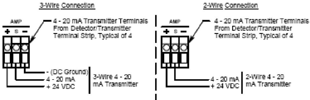
Figure 10: Generic 4 to 20 mA Transmitter Wiring
