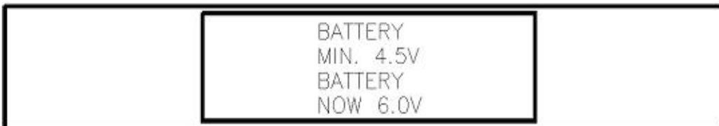
NOTE: The following screen only displays if the data logging option is installed. If the data logging option is not installed, the Self Diagnosis screen displays after the Battery Voltage screen.
