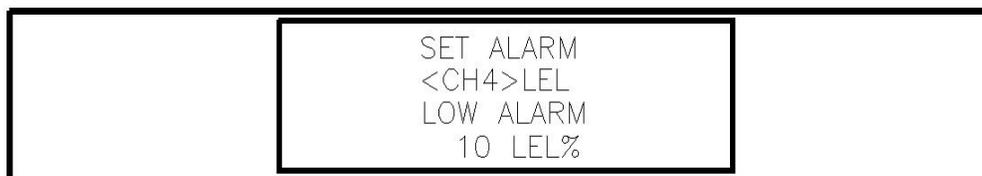
NOTE: The Gas Sniper displays the set alarm point screens for each channel in the following sequence: low alarm, high alarm, TWA alarm (toxics only), and STEL alarm (toxics only).
