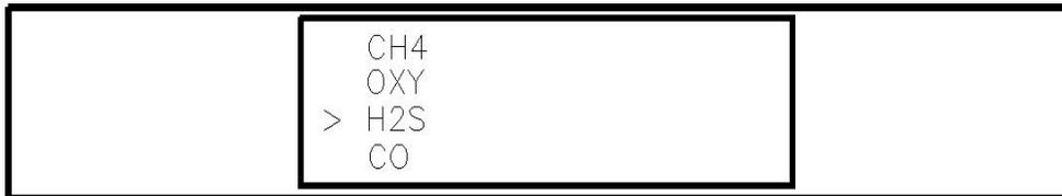
3. Use the AIR/▲ or SHIFT/▼ button to place the prompt next to the toxic gas channel (in this example H2S or CO).
