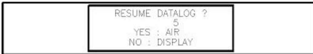
Press the AIR/▲ button to continue accumulating time-weighted average (TWA) and PEAK readings from the last time the Gas Sniper was used. (The short-term exposure limit [STEL] reading is reset each time the Gas Sniper is turned on.) The Battery Voltage screen displays.
