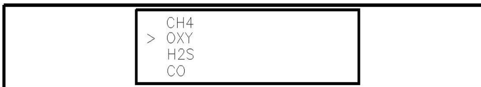
2. Use the AIR/▲ or SHIFT/▼ button to place the prompt next to the oxygen channel (in this example OXY).
