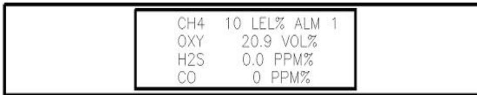
The screenshot shows a rectangular display area with a white background and black text. The text is arranged in four lines, each representing a gas channel. The first line is 'CH4 10 LEL% ALM 1', the second is 'OXY 20.9 VOL%', the third is 'H2S 0.0 PPM%', and the fourth is 'CO 0 PPM%'. The 'ALM 1' text is highlighted in a darker shade, indicating an active alarm for the CH4 channel.
