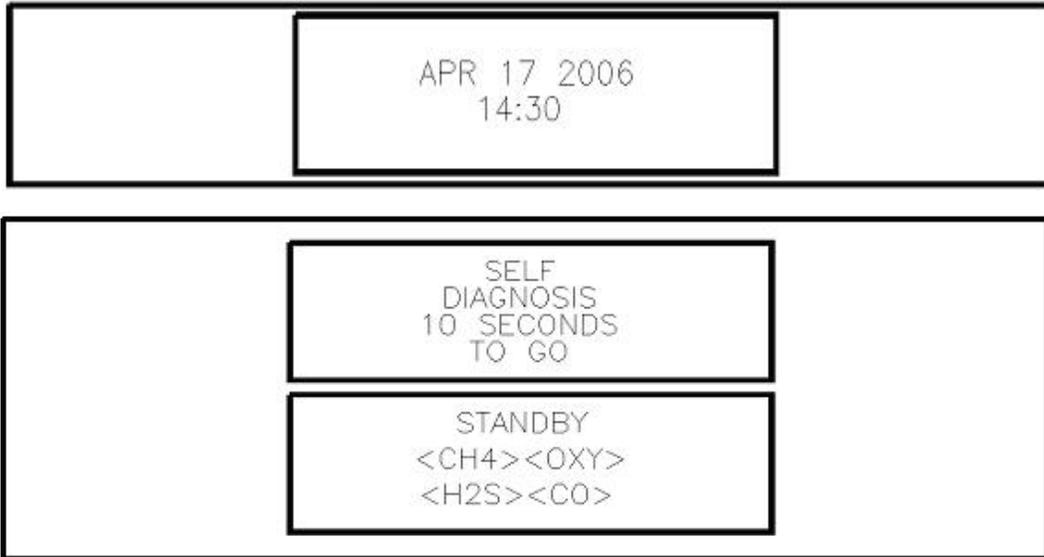
When the Gas Sniper successfully completes its self check, the **OK** message displays in place of the **STAND BY** message, then the normal operating screen displays. The normal screen displays fresh-air concentrations for all gases. The Gas Sniper sounds a double tone to indicate it is in normal operation.
