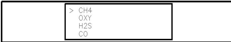
3. Use the AIR/▲ or SHIFT/▼ button to place the prompt next to the channel to calibrate (in this example the combustible gas channel).
