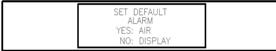
3. Press the AIR/▲ button to reset all alarm points to their default settings. The messages **SAVING DATA** and **END** display, then the main menu displays.
