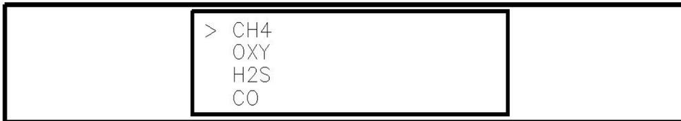
2. Select the channel of the alarm point you want to update. The channel's Set Low Alarm Point screen displays (in this example for the combustible gas channel).
