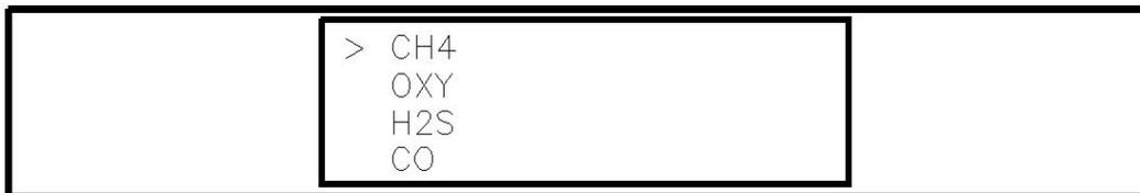
1. Use the AIR/▲ or SHIFT/▼ button to place the prompt next to the combustible gas channel (in this example CH4).
