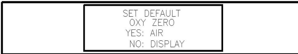
4. Press the AIR/▲ button to reset the oxygen zero setting to its default value. The messages **SAVING DATA** and **END** display, then the main menu displays.
