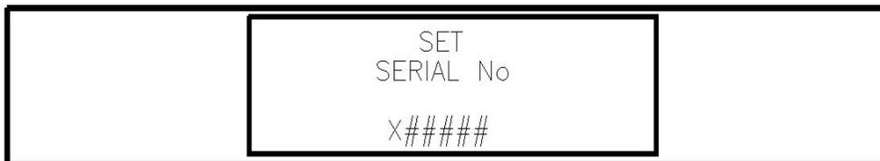
2. Press the **AIR/▲** and **SHIFT/▼** buttons to display the desired character, then press the **POWER/ENTER** button to enter the character. The next character flashes.
