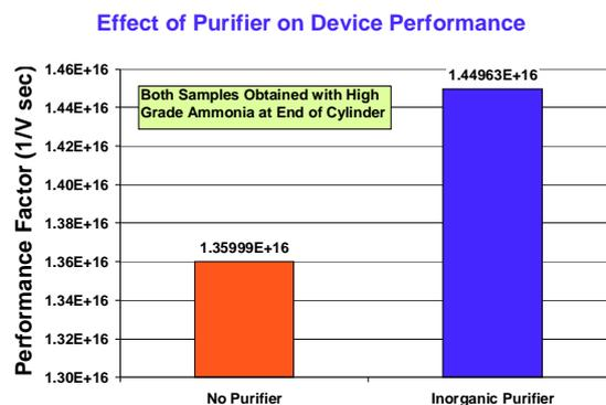
Fig. 7. Performance factor comparison for GaN device grown with an inorganic purifier compared to a device grown without ammonia purification of any kind. The devices were fabricated using high grade ammonia at the end of the cylinder.
