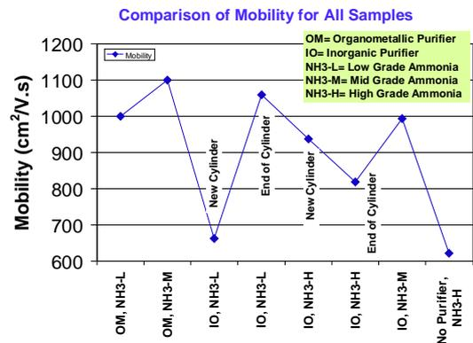
Fig. 2. Carrier mobility results for all samples included within the current investigation.
