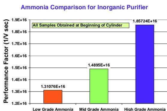
Fig. 6. Performance factor comparison of three different ammonia sources at the beginning of the cylinder while purifying with the inorganic purifier medium.
