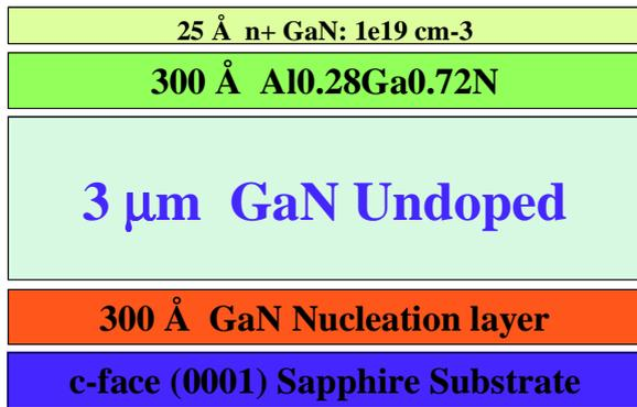
Fig. 1. Structure of devices used for all samples involved with current investigation. Schematic not drawn to scale.
