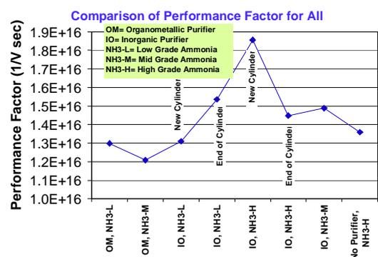
Fig. 4. Comparison of performance factor for all samples included within the current investigation. The performance factor consists of the product of mobility and sheet concentration.
