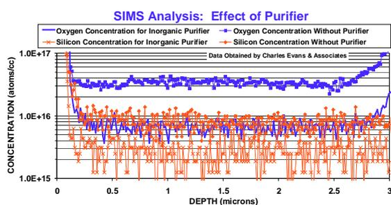
Fig. 8. SIMS results for samples fabricated with and without purification of ammonia.
