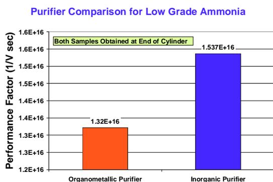
Fig. 5. Performance factor comparison of two different ammonia purifiers using low grade ammonia at the end of the cylinder.
