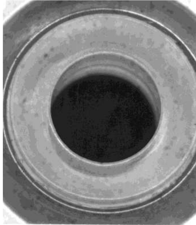
Kel-F valve seat of line valve in HBr service with Nanochem purifier, 1000 cycles
