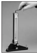
1. Loosen end seal
