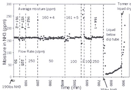
Figure 6. Moisture concentration from Matheson liquid delivery system and ammonia vaporizer while changing flow rates.
