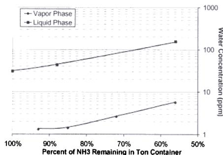
Figure 2. Change in the concentration of moisture in gas and liquid phase ammonia as a function of ammonia remaining in the BSGU during gas phase withdrawal.
