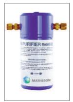
This unit will remove O<sub>2</sub> or water vapor from inert gas carriers such as nitrogen, helium, or argon to less than 1 ppm. Six (6) standard cylinders of 300 cu. ft. are easily treated where the incoming O<sub>2</sub> concentrations are 10 ppm or less.
