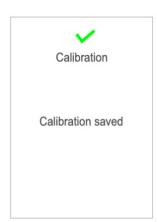
**Leak Calibration:** The calibration process for leak calibration is very similar to the calibration process for concentration calibration (ppm). The leak calibration will ask you to input the calibration gas and the name you would like to save the calibration as. The difference is that the leak calibration will ask you to input the leak rate (cc/s) of the calibration gas. Once the pump calibration is complete you will supply the probe with the known leak rate (cc/s) of the calibration gas.
