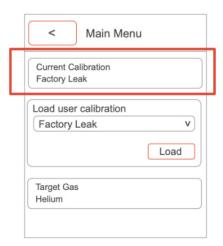
**Load User Calibration:** This option allows you to change between calibrations stored on the instrument. Once you have selected your required calibration, ensure you press load to update the current calibration.
