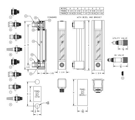
The parts listed below are applicable to MATHESON FM-1000 and FM-1050 flow meters. Recommended spare parts are indicated by \*.
