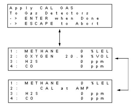
If any of the displayed channels is a 4 - 20 mA type detector head, the gas name and concentration will alternate with **CAL at AMP**. In the example above, channel 2 is a 4 - 20 mA type channel
