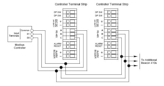
Figure 11: Recommended Modbus Wiring
