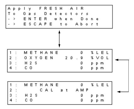
If any of the displayed channels is a 4 - 20 mA type detector head, the gas name and concentration will alternate with **CAL at AMP**. In the example above, channel 2 is a 4 - 20 mA type channel.
