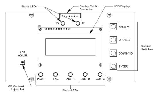
Figure 2: Control PCB Component Location
