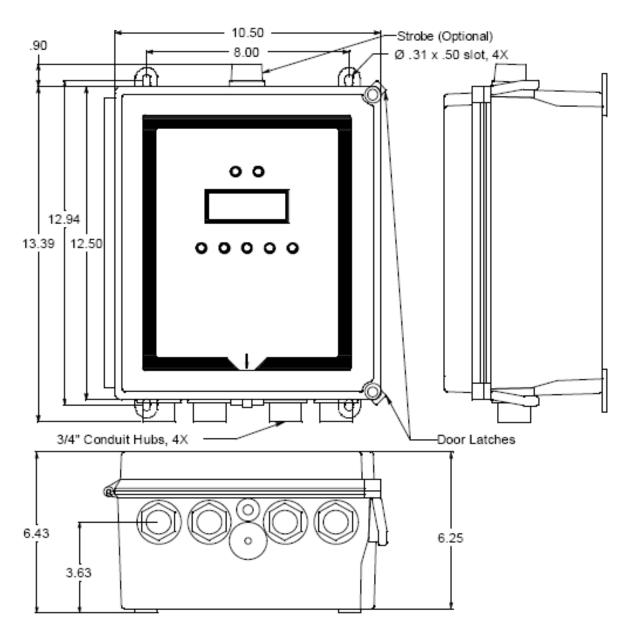
Figure 4: GasScanner 4C Gas Monitor Outline and Mounting Dimensions
