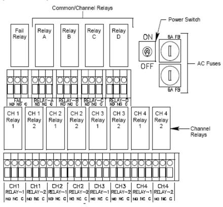
Figure 3: GasScanner 4C Relay Allocation
