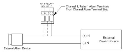
Figure 8: External Alarm Wiring
