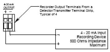
Figure 9: Recorder Output Wiring
