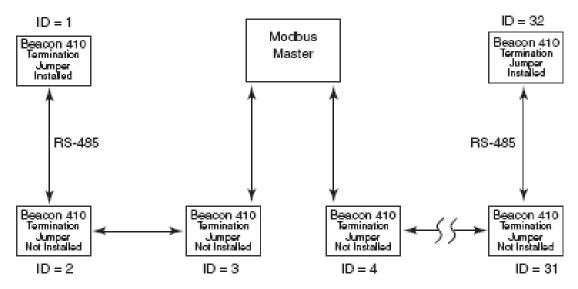
Up to 32 Beacon 410s can be connected without a repeater.
