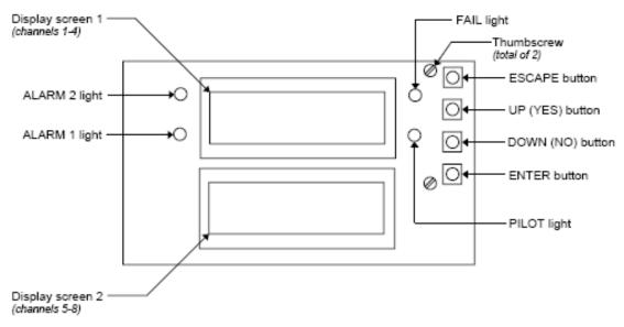
Figure 2: Display Board Component Location
