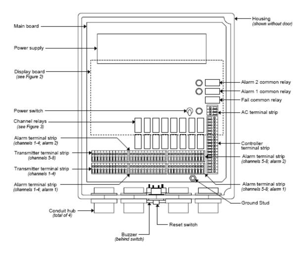
Figure 1: GasScanner 8C Gas Monitor Component Location
