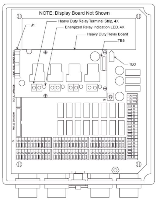
Figure 15: GasScanner 8C with Heavy Duty Relay Board
