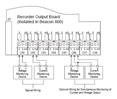
Figure 14: Recorder Output Board Wiring
