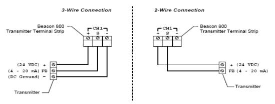
Figure 9: Generic 4 to 20 mA Transmitter Output Wiring
