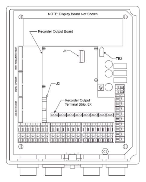
Figure 13: GasScanner 8C with Recorder Output Board
