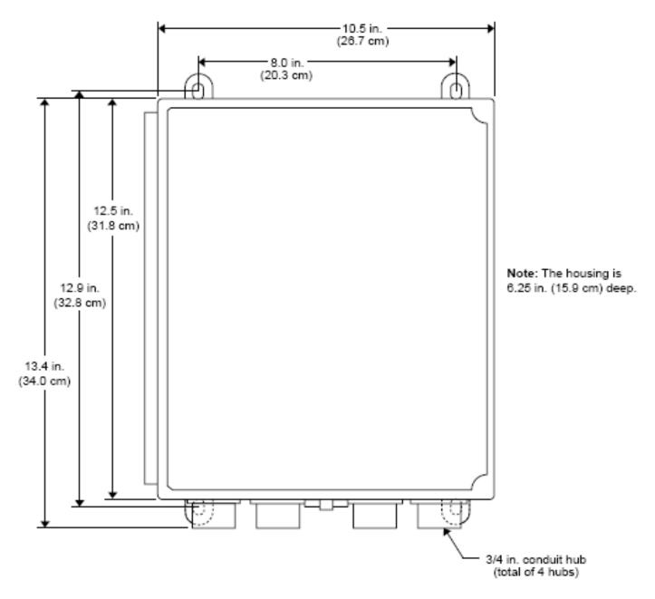
Figure 4: GasScanner 8C Gas Monitor Outline and Mounting Dimensions
