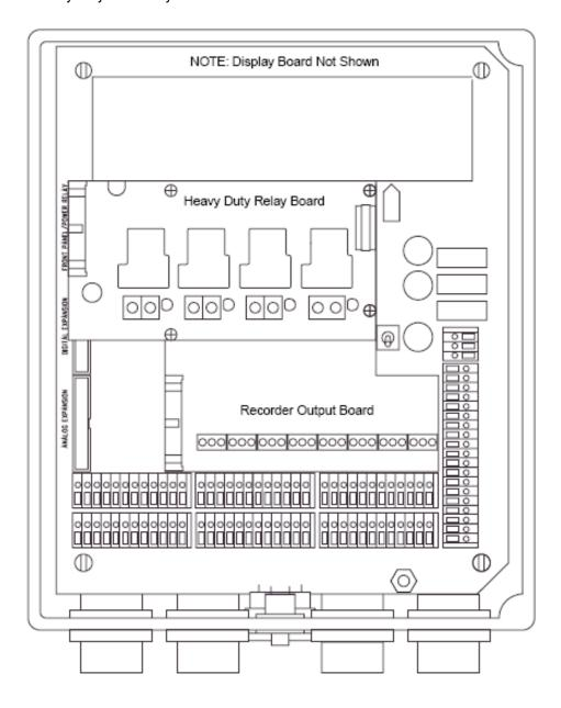
Figure 12: GasScanner 8C with Recorder Output and Heavy Duty Relay Board
