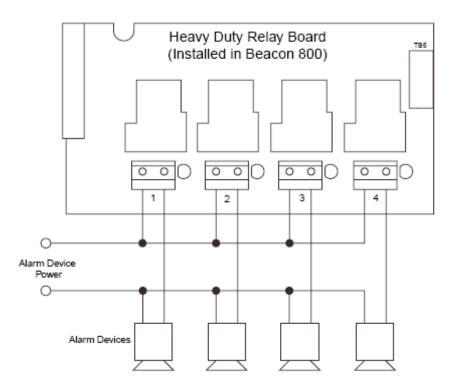
Figure 16: Wiring the Heavy Duty Relay Board
