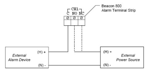
Figure 8: External Alarm Wiring
