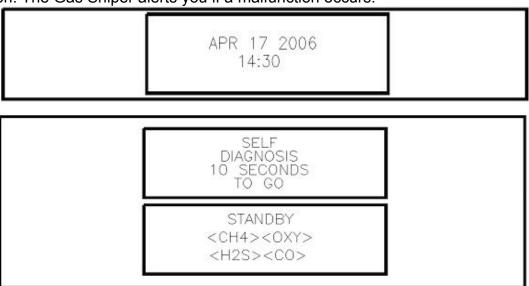
When the Gas Sniper successfully completes its self check, the **OK** message displays in place of the **STAND BY** message, then the normal operating screen displays. The normal screen displays fresh-air concentrations for all gases. The Gas Sniper sounds a double tone to indicate it is in normal operation.
