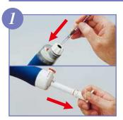
Insert a sealed, unbroken detector tube into the rubber tube connector. Align the red line on the bottom case and that of shaft, and pull the handle to full stroke locked position.
