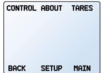
Tare mass flow by selecting TARES from the main menu .
