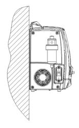
Drill appropriate holes in the wall or permanent structure and insert supplied mounting screws. Tighten only enough so there is approximately 1/4" extruding from the surface. The mounting holes are spaced 7-7/8" (200 mm) apart.
