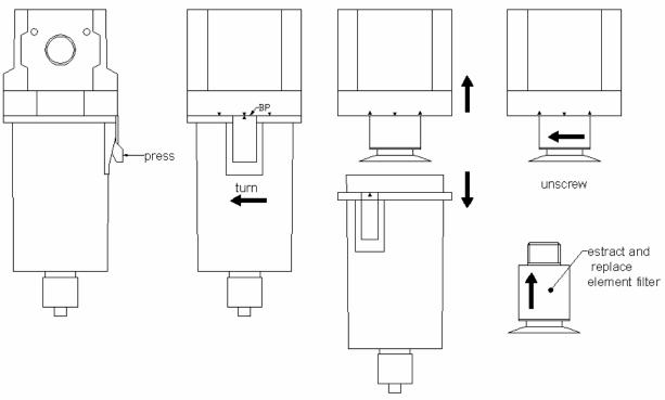
Fig. 1: Pre-filter disassembling for element filter replacement.
