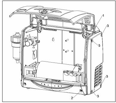
8.3.9 Carefully disconnect the two compression air fittings (1) and (2) to remove the cooling spiral (3).
