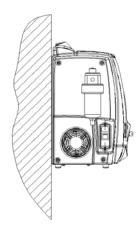
✓ Drill appropriate holes in the wall or permanent structure and insert supplied mounting screws. Tighten only enough so there is approximately 1/4" extruding from the surface. The mounting holes are spaced 7-7/8 in (200 mm) apart.
