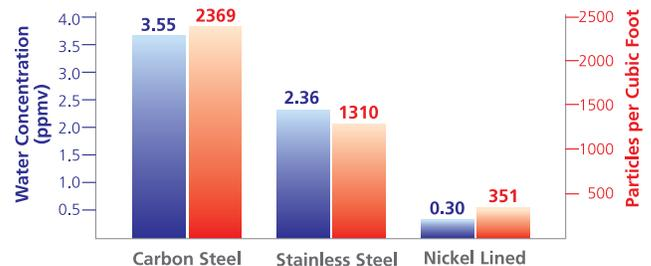
Measured shortly after fill, this comparison shows extreme improvement in contaminant reduction in the Nickel lined cylinder.
