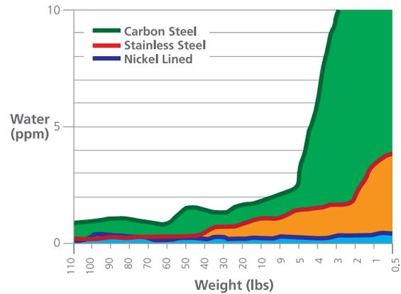
It is common practice to take a cylinder off-line before phase break (the point at which all liquid contents are vaporized in the cylinder). In this test, we ran all three cylinders (Carbon Steel, Stainless Steel, and Nickel Lined) until completely empty. Water contamination is significant in both types of Steel cylinders – even long before phase break. Water contamination in a Nickel lined cylinder is far lower, and virtually flat.
