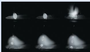
It is generally well-known that 90%He is not suitable for use with spray arc welding on stainless – these images in the series at the top help us understand why this is so. The arc plasma has a noticeable plasma shift; droplet formation is large and the transfer is explosive. The lower series of images demonstrates the suitability of HC-725 for spray arc welding. Droplet formation and transfer are smooth and consistent; and the plasma is stable.
