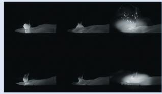
Note the large droplet formation, globular puddling, and explosive spatter in the upper series where 90%He / 7.5%Ar / 2.5%CO<sub>2</sub> was used. In the lower series (using HC-725 as the shielding gas), the droplet is smaller and puddling is smoother, giving the user better overall control (and a better appearance). In addition, re-ignition of the arc with HC-725 is less explosive, causing less spatter.
